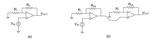
**Problem 9** Two operational amplifiers are shown below. Assume the standard symmetry properties in both structures.
